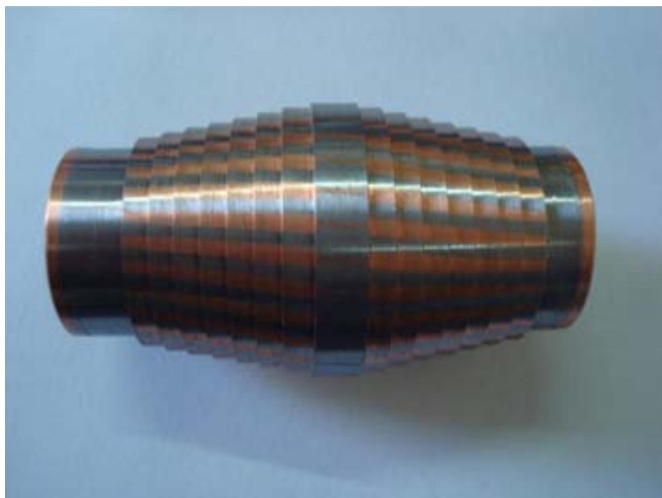
Figure 1, internal quality of cast copper rotors
