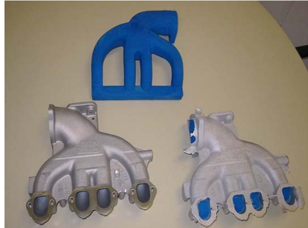
3 Intake manifold casting using Cordis binding system (core is shown on top) 39
