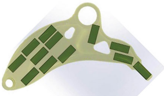
Fig. 1 Control arm and the location of the cut coupons. (Color figure online)
