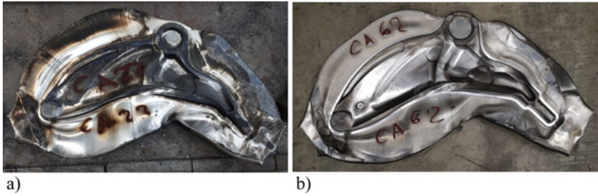
Fig. 5 ZK60 control arm forgings at a 450 °C and b 300 °C. (Color figure online)
