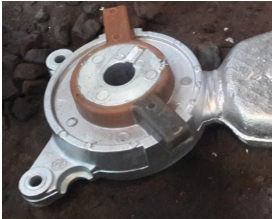
Figure 12. The casting part with salt core that comes out of the casting mold.
