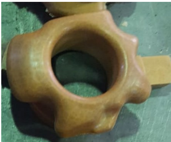
Figure 10.2. Salt core produced in high temperature and long time.
