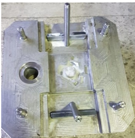
Figure 2.1. Injection mold movable side manufactured for salt core
