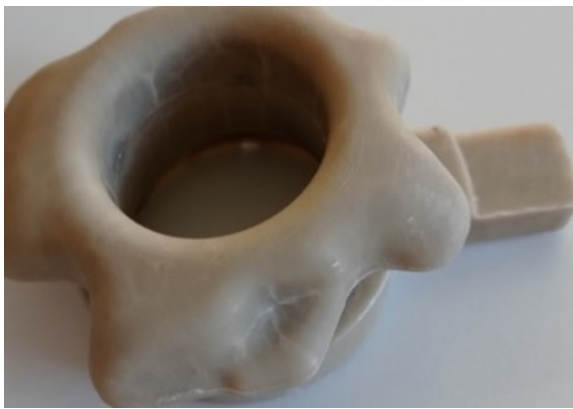
Figure 10.1. Salt core produced in low temperature and short time.
