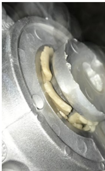
Figure 13. The salt that starts to dissolve, the core and the cast part.
