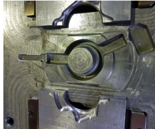
Figure 2.2. Injection mold fixed side manufactured for salt core.
