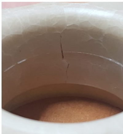
Figure 6. Salt core inner diameter surface crack visible with eye control.
