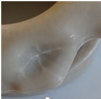
Figure 5. Salt core exterior surface crack.
