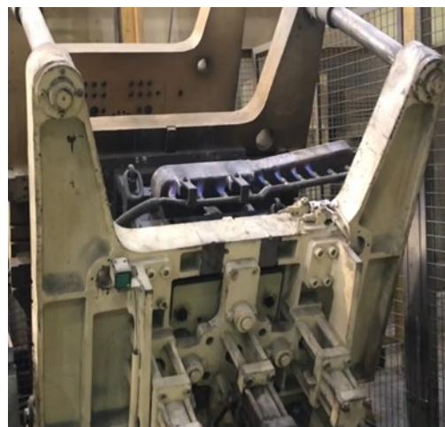
Figure 11.3. The tilt casting machine rotates 180 degrees.
